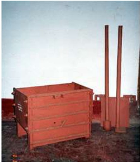
Rammed earth technique developed by Mrinmayee Bangalore Earth is rammed in a smaller blocks of 2 feet length, using formwork which can easily be installed and shifted to adjacent sections of the wall
